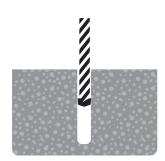
With the correct diameter drill bit, drill a hole to the correct depth.
