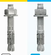
ICCONS® THRU-BOLT is a pre-assembled a torque controlled mechanical stud anchor, which when tightened draws the tapered end of the bolt into the expander clip expanding it to create expansion forces against the wall of the hole.
